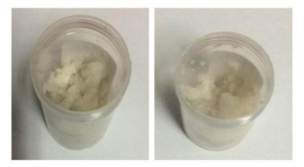
Figure 2. Extracted cellulose from *Suwandel* (left) and *Raththal* (right) rice straw varieties
