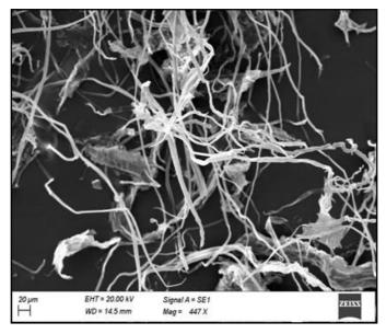
Figure 4. SEM Micrograph of cellulose extracted from Suwandel Rice Variety
