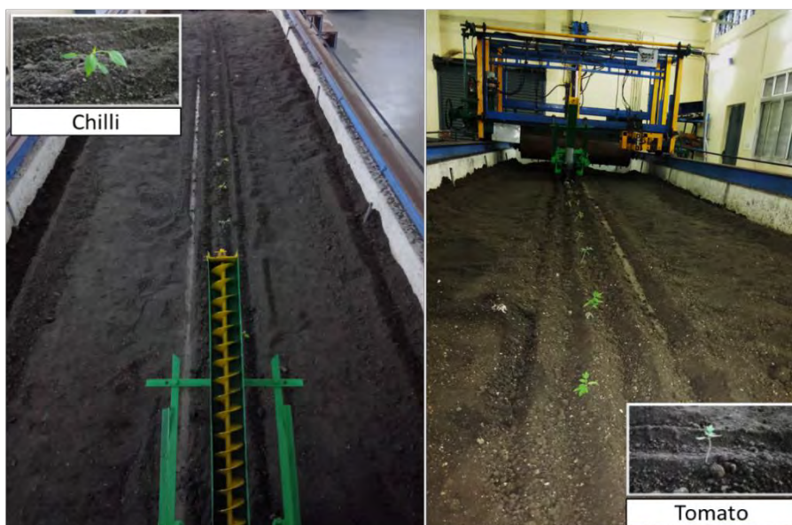
Figure 3. Pictorial views of seedlings fed to the metering unit (inset) and transplanted seedlings by the developed auger conveyer type metering unit in the soil bin condition
