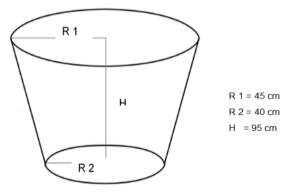
Figure 3. Dimensions of broodstock tanks
