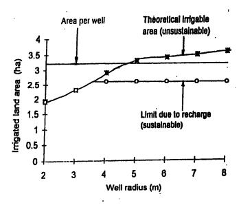
Figure 2. Effect of well radius on irrigated land area with an aquifer depth of 6 m and well spacing of 180 m.
